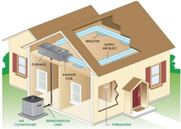
split systems (ducted)
