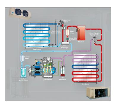
This Testo program is for the HVAC professionals who want to learn more about the Pressure/Temperature Relationships in AC, Refrigeration systems, and how to correctly measure the performance of the system by looking at Superheat and Sub-Cooling. The course offers a better understanding of the refrigeration cycle, its components, and analog gauges vs. digital manifolds. It will provide a collection of knowledge in the Laws of Refrigeration and Heat Transfer.
